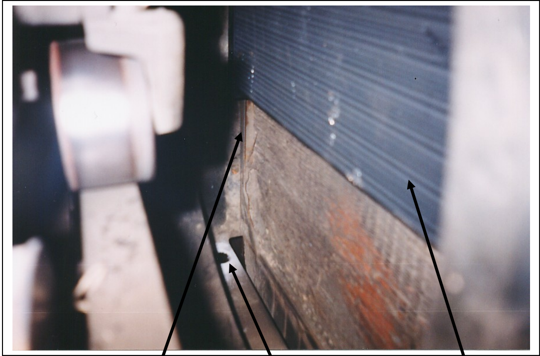
Condenser bolts to threaded holes on radiator flange
